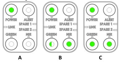
the GREEN and NIR LEDs should turn green to indicate that both lasers are switched ON. If any of the laser LEDs is blinking green, this means the laser source needs time to reach nominal temperature (few seconds to 3 minutes) before firing [B].
