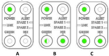
GREEN and NIR LEDs should turn green to indicate that both lasers are switched ON. If any of the laser LEDs is blinking green, this means the laser source needs time to reach nominal temperature (few seconds to 3 minutes) before firing [B].
